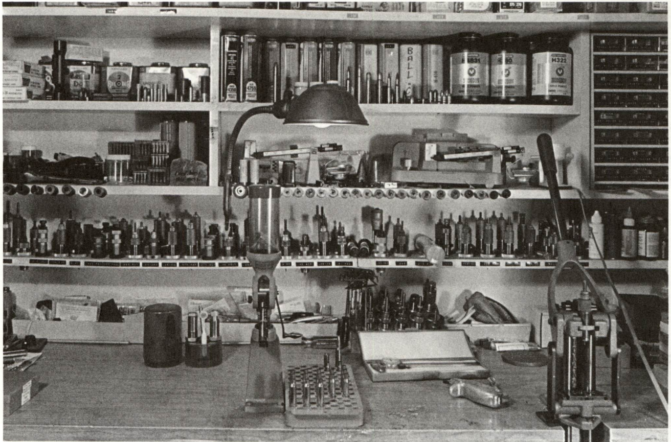
A well-equipped reloading bench is a small ammunition factory. Here you can assemble the specialized cartridges for any kind, caliber, or gauge of firearm.
