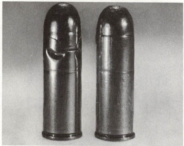
Insufficient flare on the mouths of straight-sided revolver cases often results in crumpled and ruined cases during the bullet-seating step.
