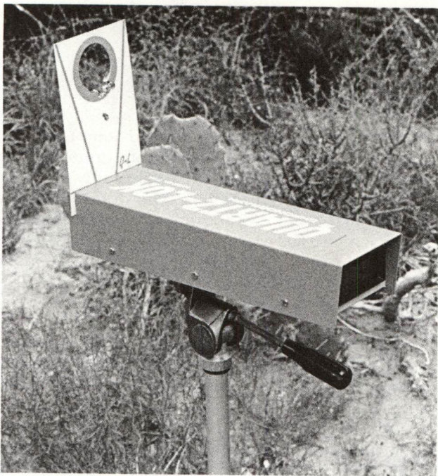
The all-in-one-unit Quartz-Lok chronograph offers the simplest imaginable setup with permanently spaced optical screens. The liquid crystal display readout gives velocity only.
