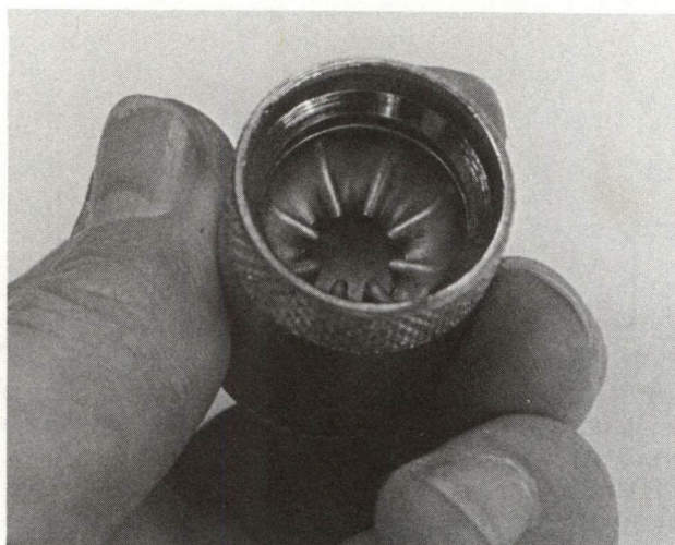
Crimp-starters come in six- or eight-point models. This is an eight-fold starter. The more sophisticated tools are self-indexing.
