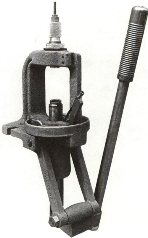
Left: The RCBS "Rockchucker" is a classic example of the "O"- (or "D"-) frame metallic press. Right: This is Lee Precision's lightweight "O" press.
