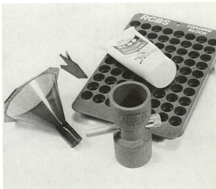
Left: This Belding and Mull powder measure, long popular with benchresters, is not only unique in principle but is also one of the oldest reloading tools still in manufacture. Right: Essential small tools and accessories include (clockwise from left) powder funnel, chamfer-deburring tool, loading block, primer-pocket cleaner, and powder trickler. A tube of resizing lube rests upon the loading block.
