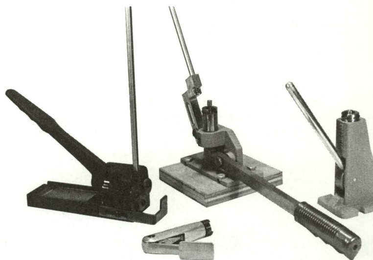
A few of the special priming tools available are, from left, Bonanza, Lee, and two RCBS models.
